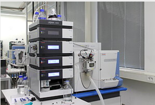
Orbitrap Elite (Thermo Scientific) mit UHPLC (UltiMate 3000, Thermo Scientific)
