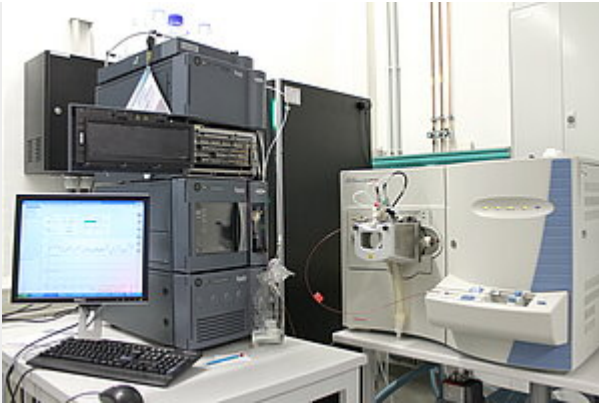
ESI-Ion-Trap-System (Thermo) mit UPLC (Waters Acquity)
