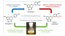
Process for the production of HED. The enzymes suitable for the two-stage conversion of naringenin into HED were identified by rational design or activity screening (upper part). These could then be used to produce the bitter-masker in the whole cell system (lower part).
